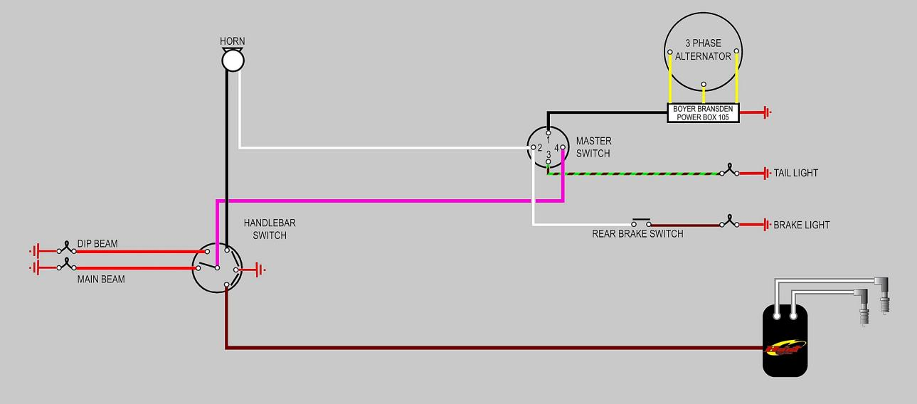
Removed factory points, condenser and ballast resistor
