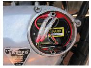
Connect the black/white and black/yellow wires as shown in the photograph above forming the wires in a bend to reduce the strain on the wires caused by vibration.
