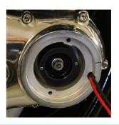
Install the Tri-Spark rotor using the correct socket head bolt for your engine. Two are provided (1/4 UNF and 1/4 BSF) for use with the earlier and later engine models. When tightening the bolt ensure correct torque and check the fit of the taper inside the cam.
