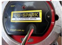
Mark the engine casing adjacent the "CW" line on the outer rim of the stator unit, then remove stator unit.
