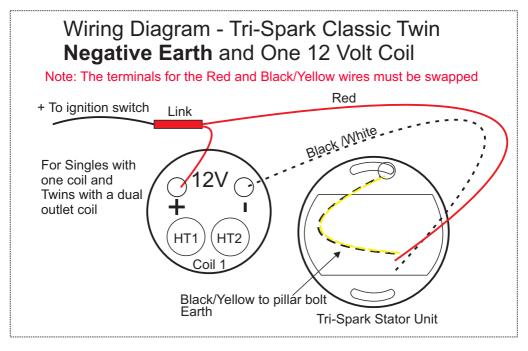
Note: 'To ignition switch' means make connection with the wire intended for switching the ignition on/off at a convenient point. This is often a white/yellow wire that was originally connected to the negative side of the ignition coil(s) when running on points. Normally this connection is switched by the ignition and kill switches.
