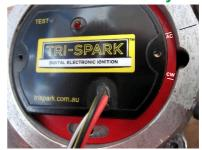
Mark the engine casing adjacent the "AC" line on the outer rim of the stator unit, then remove stator unit.
