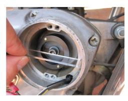
Install the stator unit using the original pillar bolts and washers. Use additional washers if the pillar bolts bottom out. Do not tighten the pillar bolts at this time - adjustment will be made later on.
