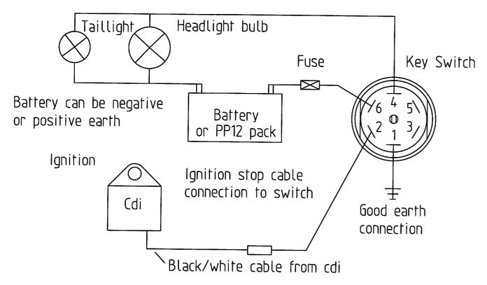
Contact arrangement as shown below is with the ignition OFF The key is removable in this position.
